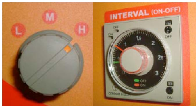
**Figure 2: The output selector switch (left) and interval control knob (right)**
