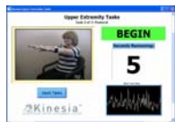
Figure 2. The Kinesia software uses clinical videos to automatically guide patients through motor tasks while motion data are recorded.
