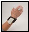
Figure 1. Kinesia™ consists of a finger worn sensor unit that contains three accelerometers and three gyroscopes, and a wrist worn command module that wirelessly transmits data to a computer.
