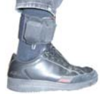
Fig. 1. Ambulatory gait monitor, consisting of an IMU, bluetooth transmitter and battery.
